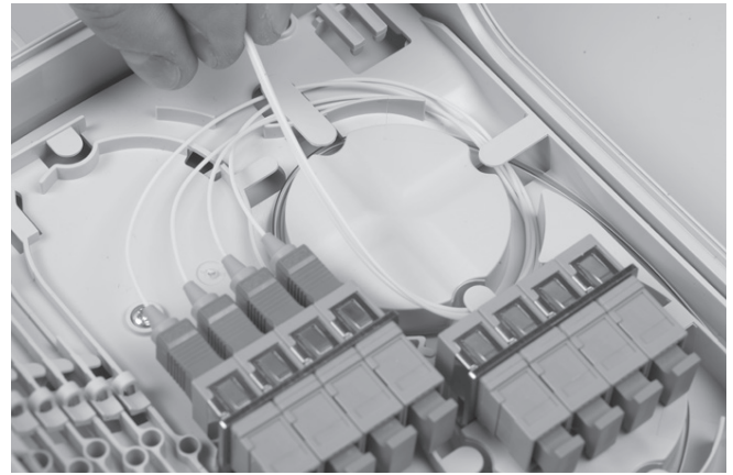
4.4 Connect first four 900µm pigtails.
