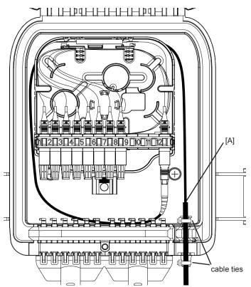
9.3. If a breakout (for a flat cable for instance) or a stripping point on the cable is present [A], make sure it is inside the terminal for proper protection.
