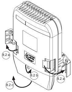
8.2. Then open the terminal by releasing the latches (a), rotate the locking bolt counter clockwise (b) and lift the top cover open (c) until its lock position.
