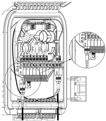
10.1. Remove the dust caps, clean the connector per standard practice and mate the connector to the adapter in its assigned port (numbers 1-8). Verify the correct orientation as shown above. You will hear a clicking sound when the connector is properly seated. Page 3 © 2017 Commscope
