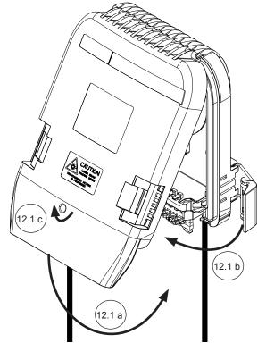
12.1. Swing the cover down (a), close the latches (b) and lock the bolt by turning the Phillips screw driver CW.
