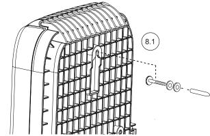
8.1. First install the central screw and hang the terminal on this screw. Use the metal washers from the kit content.
