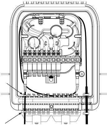
10.2. Secure the drop cables with the cable ties. Secure them inside and outside.
