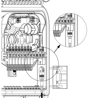
9.1. Remove the dust caps, clean the connector per standard practice and mate the connector to the adapter in port 12. Verify the correct orientation as shown above. You will hear a clicking sound when the connector is properly seated.
