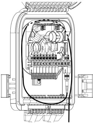
9.2. Make a loop with the feeder cable around the spool before exiting the terminal. One loop is approximately 0.5m (20"). More then one loop around the spool can be made if some slack storage is required. Mind proper minimum radius bend of 30 mm (1.2").
