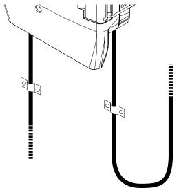
12.2. It is recommended to anchor the flat cable (feeder cable or drop cable) to the wall with a small clip.
