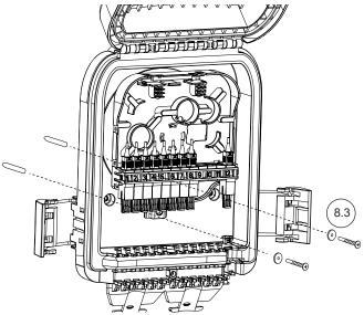
8.3. Make a hole through the plastic on the location of the mounting features inside the terminal and make a mark on the wall through these holes. Take off the terminal and drill the 2 holes, install the plugs. Hang the terminal again on the first screw and secure the two other screws. Use the plastic washers from the kit content.
