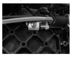
5.14 Fix the cable at the cable ports by black tie wrap and remove the spare length.
