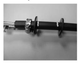
5.9 Tear off the gel strip and wrap it between the two rings. Press the opening of gel strip firmly while start and finish to ensure the gel strip flat and no pulling during wrap.
