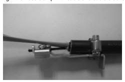
5.4 Select the ring with the hole's size a little bigger than cable diameter and take it off.
