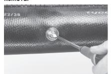
1 Remove the valve plug or the core valve.
