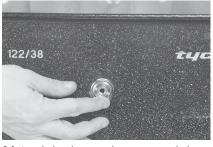
**14** Attach the sleeve to the canister with the valve nut and hand tighten.
