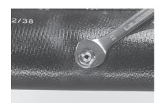
**25** Allow the sleeve to cool down undisturbed for at least 15 minutes. Tighten the valve nut.
