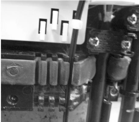
10.9 Close the lid, screw the center screw and latch the top cover, as shown.
