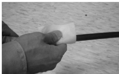
5.3 Fix the strength member underneath the metal screw as shown in **Step 5.4**. Tighten the screw to secure the strength member. Cut the excess off.
