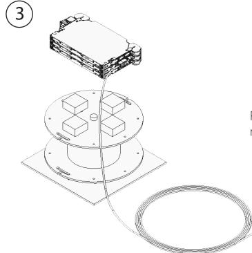
Remove the straps. Unpack the elements and mount them in the frame.
