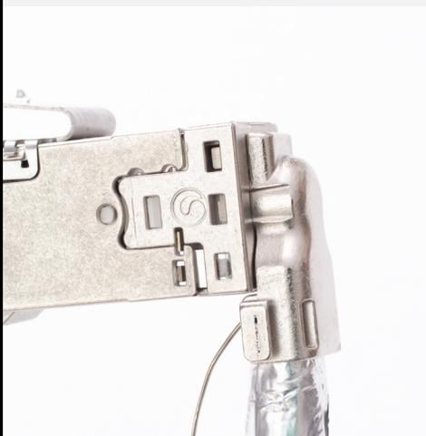
Step 8 – Position drain wire, if present, to contact cable clamp.
