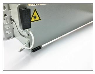
10.1.6 Option; to secure the cover together with the panel (when taken of) install a rope between the cover and shelf. (Not included in the standard kit)
