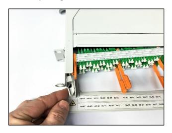
10.4.1 Open one subunit by pressing the locker insides and slide open the subunit.
