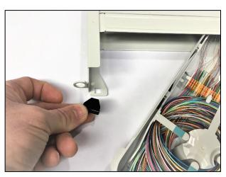
10.1.2 Open the subunit and place the hinge on the left side.
