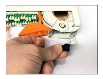
10.1.1 Install the hinge on right side of the shelf by first inserting the narrow end of the hinge into the hinge slot and then snap it into place.
