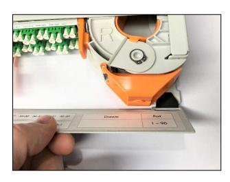
10.1.3 Take the front cover, place it into the slot of the hinges under an angle of 45°, push until the cover is fixed. Repeat on the other side.
