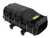
OFDC B8G Fiber Optic Splice/Patch Closure, Gel Cable sealing, 6 preinstalled 12 fiber trays , 8 duplex LC/APC adapters, 1-8 splitter pre-conn at drop side
