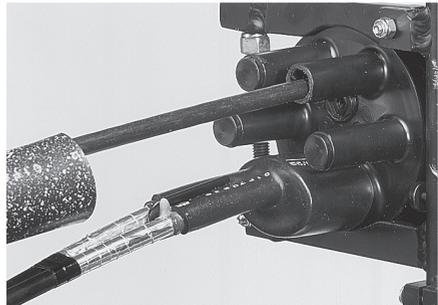
11.5 Align cable ring cut with the edge of the base. Slide strength member into clamp and tighten the nut. Cut away the excess length of strength member.
