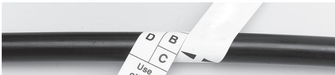
1.1.3 Measure the cable(s) with the tape supplied in the kit to determine the appropriate branching plug/port to be used.
