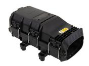
OFDC B8G Fiber Optic Splice/Patch Closure, X-press version, Gel Cable sealing, 1 pre-installed 18-fiber splice tray, 8 duplex LC/APC adapters, 20 m drop cable assy, mobra
