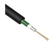
Fiber OSP cable, 24-fiber, OS2, HDPE, loose tube, 24 fiber, gel-filled, Singlemode G.652.D and G.657.A1, 1000 m, Meters jacket marking, Black jacket color
