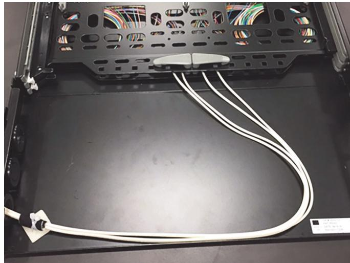
9. Now add the split grommet back around the cable (removing the center plug from it) and push all plugs back in place.
