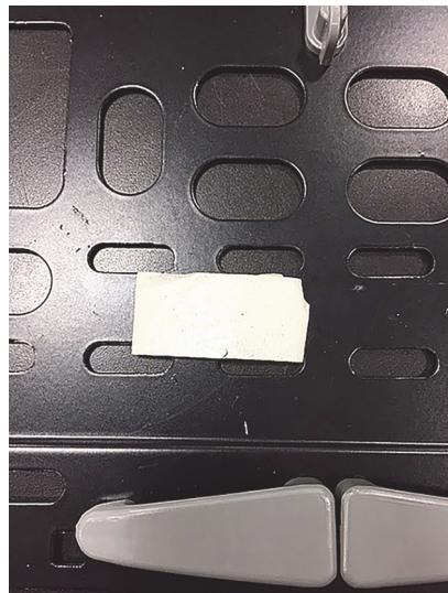
3. Route the fibers through the rear side hole on the side you want to enter the panel. Populate both the adapter packs with the fanned-out fibers. Move the fanout so the 3mm cable tails go under the gray tab on the side you are populating and stick them down to the double-sided tape just ahead of the gray fiber managers.
