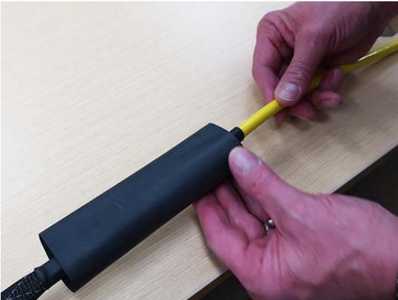
14. Shrink the large tubing using the lowest effective heat setting on the heat gun. Apply uniform heat around and across the heat shrink, using special care to prevent extreme differences in diameter. Uneven heating will cause trapped air pockets and/or backwards curling at the ends. The heat shrink is adhesive lined so it is normal to see a small amount of adhesive leaking out at the edges of the tubing.
