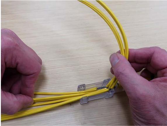
15. At a point about 1/8 inch-1/4 inch (3 mm - 6 mm) outside the fanout base, apply the adhesive generously to the first horizontal row of furcation tubes. Ensure that the application of the adhesive occurs between all the tubes. Do not allow adhesive to dry before starting Step 16.
