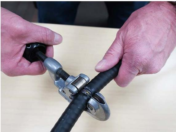
3. Slide the cable armor off of the cable.
