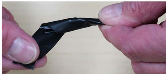
24. Slide the mesh sleeve over the fiber ribbons/furcation tubes until the end of the mesh reaches the fanout assembly, as shown in the second photo.
