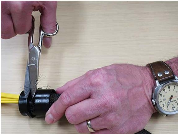
24. The cable assembly is now ready for splicing or connectorization.
