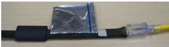
8. Wrap the foil tape around the mesh sleeve, making a minimum of 1-1/4 revolutions.
