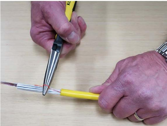
9. Pull the ripcord(s) to split the cable sheath back to the ring cut at the 96-inch (244 cm) mark. Needle nose pliers can be helpful to grasp and pull the ripcord(s).
