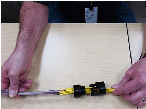
19. Slide the end of the mesh sleeve into the gland cap.
