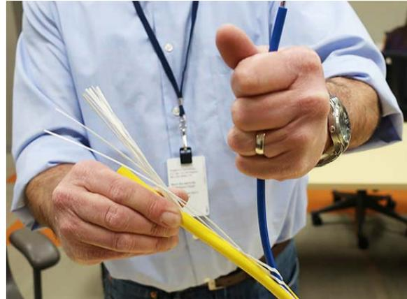
11. Remove the cable sheath, strength members, tape liner(s), and ripcord(s) at the ring cut, leaving just the central tube.
