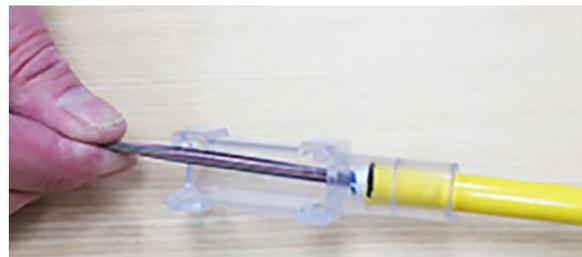
**Note:** The base should fit very snugly around the cable sheath. If necessary, make one or two wraps of electrical tape around the cable sheath to ensure a snug fit.
