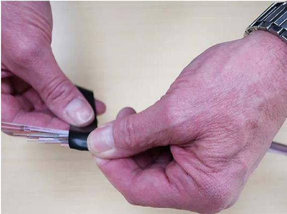
23. Wrap the tape around the ends of the fibers as shown.
