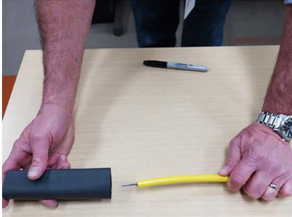
2. Slide the 6-inch (15.2 cm) heat shrink tubing up the cable and out of the way.
