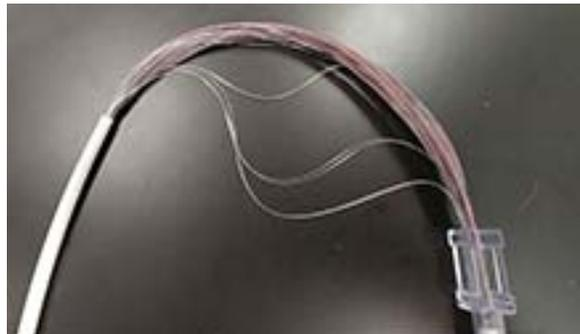
7. Identify a numbered fiber ribbon and feed the ribbon into the associated furcation tube at the 45 degree cut. The ribbon may be cleaned with an alcohol wipe prior to insertion into the tubes if desired to aid in the insertion process, although this step may be unnecessary.
