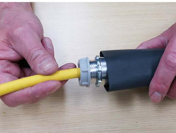
10. Using the most effective distance and lowest effective heat setting on the heat gun, shrink the heat shrink tube until it is fully compressed.
