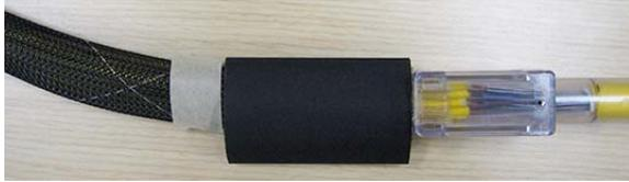
4. Slide the heat shrink a minimum of 8 inches away from the plastic fanout assembly.
