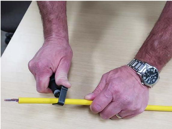
8. Remove the sheath exposing the ripcord(s) at the stub end of the cable.
