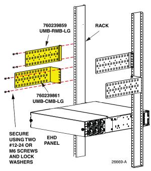
If installing a non-armored cable, secure the cable to bracket using cable ties.
