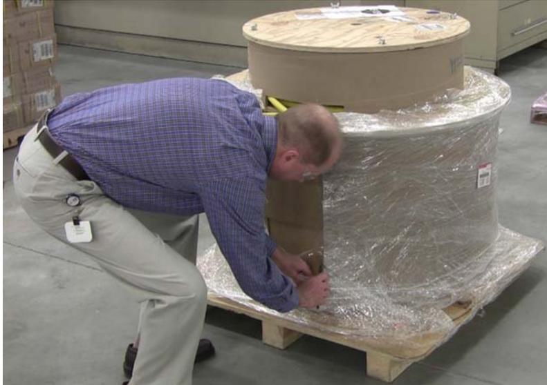
Figure 3. Cutting Off External Plastic
