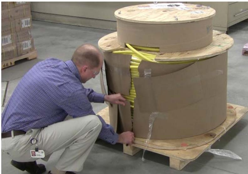
Figure 4. Cutting Off Cardboard Wrap
