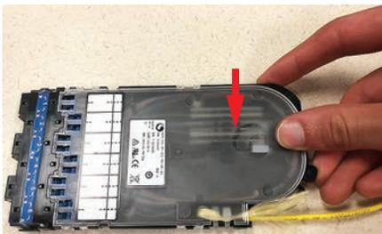
**Caution:** Prior to re-installing cover, carefully inspect routing to ensure all fibers are secured below retaining tabs and that fibers do not extend onto the ledge designated for the cover.
