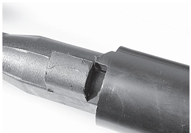
3.7.4 Tighten the trigger until it butts. When necessary, use wrench (n° 12) to tighten the trigger.
