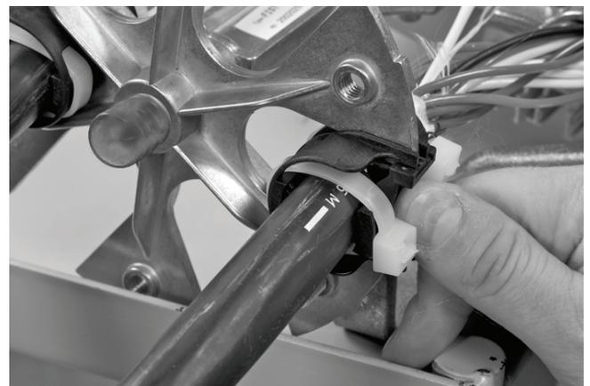
3.6.4 Slide the base over the cables and position the cable retention devices in the cable attachment plate.
