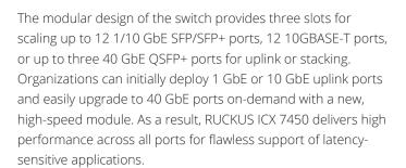
System-level high-availability features, such as dual hotswappable, load-sharing, and redundant power supplies, and hot-swappable fan trays offer another level of availability for the campus wiring closet, all in a 1 RU form factor.
