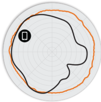
Figure 2. R310 2.4GHz Azimuth Antenna Patterns
