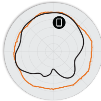
Figure 3. R310 5GHz Azimuth Antenna Patterns
