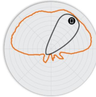
Figure 5. T811 5GHz Elevation Antenna Patterns
