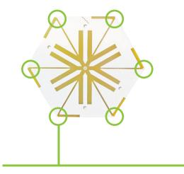
Six high-gain directional antenna elements controlled by an expert software system that determines the best antenna pair for any packet at any given time
