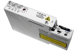
The transmitter supports Service Group Aggregation (SGA), or Daisy Chaining, with improved Noise Power Ratio performance due to advancements in A/D technology. In this process, signals from service groups—up to four nodes—are digitally multiplexed at each node and fed upstream to the master node. SGA preserves CMTS ports and RX slots in the hub or headend, providing the flexibility to expand the service group later in response to increased bandwidth demands.
