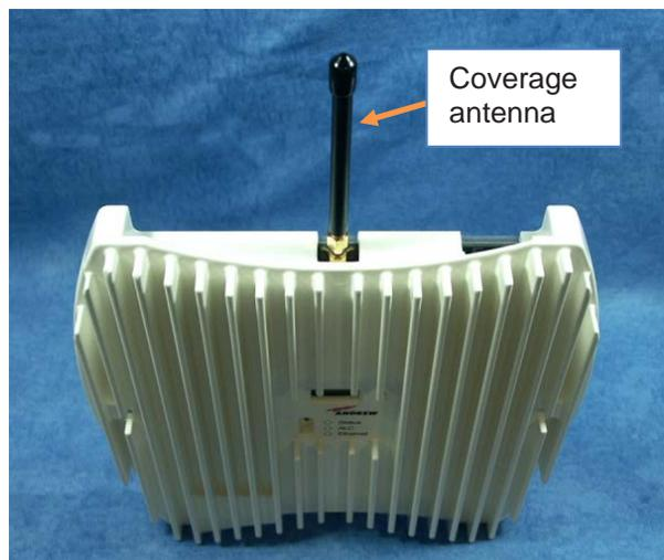
figure 6-1 Coverage antenna for MRx18, optional equipment
