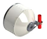
0.9m | 3ft Sentinel® High Performance Antenna, dual-polarized, 21.200 – 23.600 GHz, PBR Flange, White Antenna, Grey Radome
