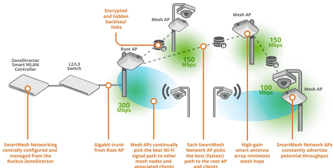
Figure 1. SmartMesh Networking with wireless video surveillance cameras
