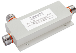
ValuDAS™ 13 dB, Air Directional Coupler, 578–3800 MHz, 4.3-10
