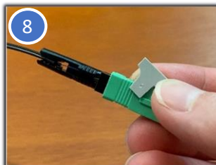
(8) Remove the aid clip from the connector, locking the splice in place. Save the clip to reuse the connector later.
