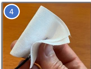
(4) Clean the fiber with a lint free wipe moistened with fiber optic cleaning fluid. Check the fiber integrity by bending the stripped end slightly at 30°
