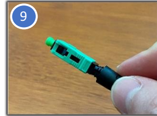
(9) Straighten the fiber, taking care not to pull back on the fiber. Thread the boot onto the back of the connector until hand tight. Termination is complete.
