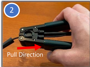
(2) Strip the jacket to 50mm using the drop cable stripper
