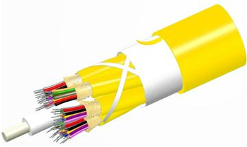
Fiber indoor cable, Low Smoke Zero Halogen Distribution, 72 fiber multi-unit, Singlemode G.657.A1, Meters jacket marking, Yellow jacket color
