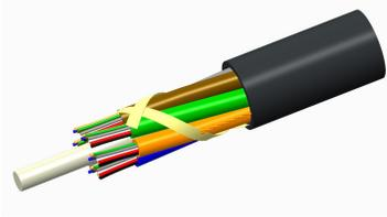
Fiber OSP cable, Zero Water Peak® Blown Micro Single Jacket, 96 fiber, All-Dielectric Outdoor Stranded Loose Tube 200um Fiber Arid-Core™ Construction, Singlemode G.652.D, Gel-filled, Meters jacket marking, Black jacket color
