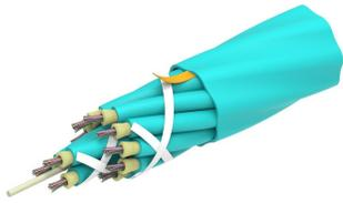
Fiber indoor cable, LazrSPEED® Low Smoke Zero Halogen Riser MPO Trunk Cable, 192 fiber with 16-fiber, 3.0mm subunits, Gel-free, Multimode OM4, Feet jacket marking, Aqua jacket color, B2ca flame rating
