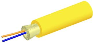
Fiber Indoor Cable, Low Smoke Zero Halogen Riser Light Duty Interconnect Cable, 2 fiber, gel-free, singlemode G.657.A2/B2, feet jacket marking, yellow cable jacket color
