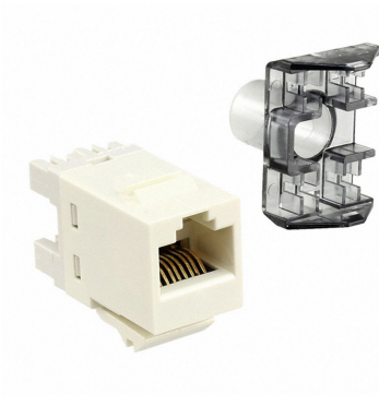
SL110 Series Modular Jack, RJ45, category 6, T568A/T568B, unshielded, without dust cover, white
