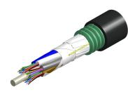
Fiber indoor/outdoor cable, TeraSPEED®, Single Jacket/Single Armor, 90 min Fire Survival, Low Smoke Zero Halogen (LSZH), 48 fiber, Singlemode G.652.D and G.657.A1, Gel-Filled, Stranded Loose Tube, Black jacket color, Meters cable marking
