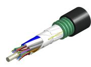
Fiber indoor/outdoor cable, TeraSPEED®, Single Jacket/Single Armor, 90 min Fire Survival, Low Smoke Zero Halogen (LSZH), 36 fiber, Singlemode G.652.D and G.657.A1, Gel-Filled, Stranded Loose Tube, Black jacket color, Meters cable marking
