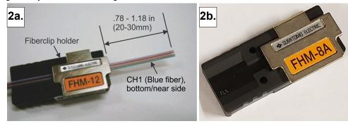
3. Place the fiberclip holder with ribbon fiber into the thermal jacket remover and close both doors. Allow stripper to reach temperature before stripping. When the heater stops blinking, it is ready to strip.
