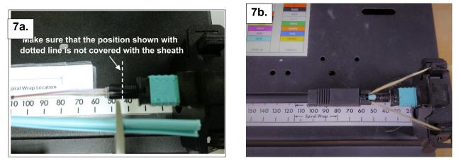
7. a: Trim the jacket up to the slotted edge (dotted line) as shown. Do not trim too short. The jacket should rest in the slotted area of the rear housing.
