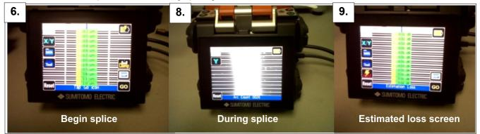
After the splice is complete, estimated results will display: green for passing, red for failing. Open the door and remove the assembly from the fiber clamps.
