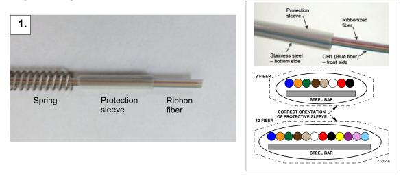
1. Using the ribbon fiber to be terminated, slide the spring and the protection sleeve from connector kit onto ribbon fiber as shown.
