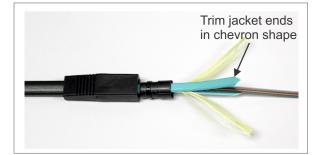
b: While holding the strengthening yarn and jacket tightly together, evenly distribute the yarn, place the jacket into its slot and slide the boot assembly up against rear housing.
