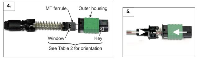
5. Snap outer housing onto the end of the rear housing. Slide the outer housing over the ferrule and spring, snap onto the end of the rear housing.
