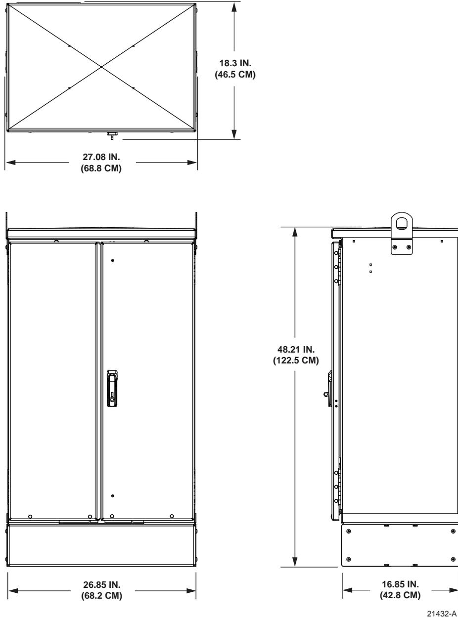
Figure 2. 432 Termination FDH 3000 Pedestal-Mount Cabinet Dimensions
