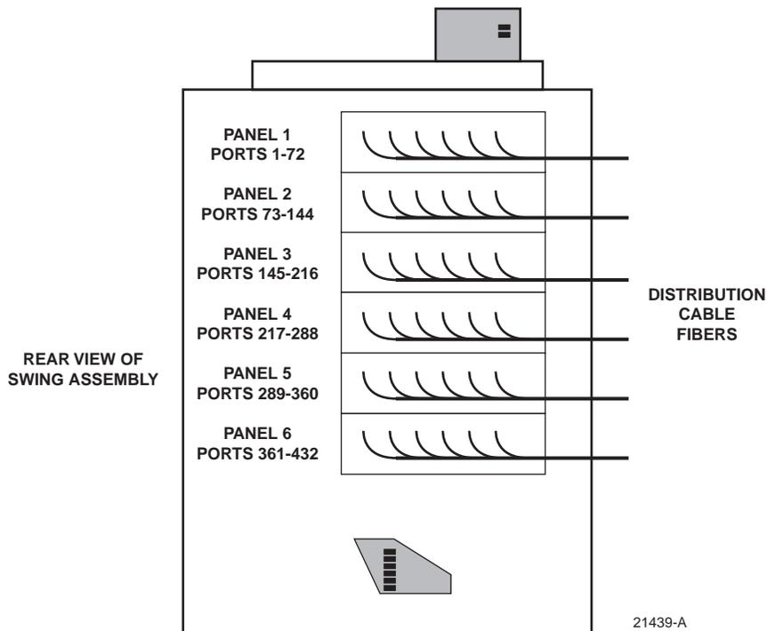
Figure 16. Distribution Cable Configuration
