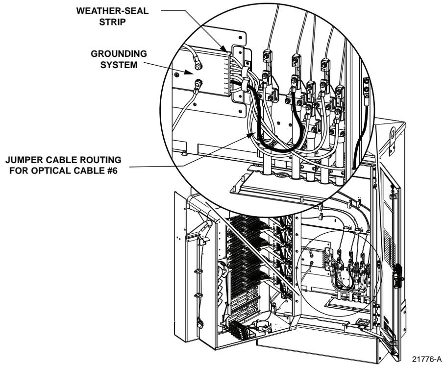
Figure 25. Cable Grounding System - Interior View
