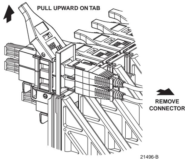
**Figure 31. Typical Adapter Pack Raised to Access Position**
