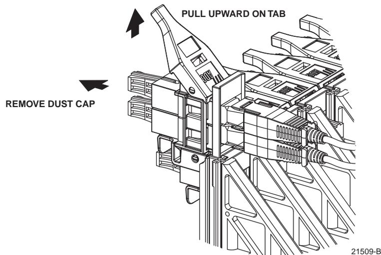
**Figure 28. Typical Adapter Pack Raised to Access Position**
