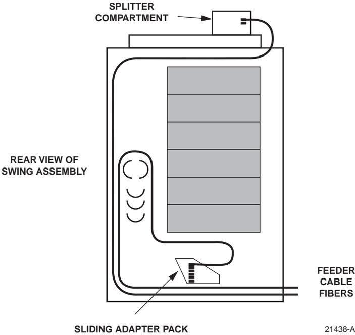
**Figure 15. Feeder Cable Typical Configuration**
