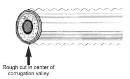
**2** Remove Jacket. Measure 1" (25.4 mm) back from the end of the cable and remove the jacket as shown below.
