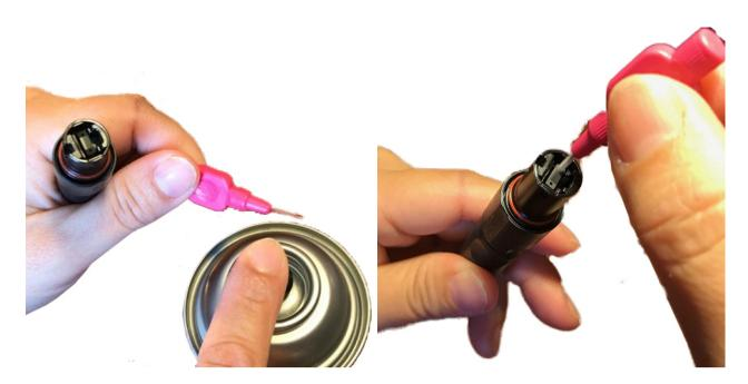
Wet the pink (0.4 mm) TePe brand dental (pinhole) brush with MicroCare FCC2 connector cleaner or equivalent cleaning solution and insert the brush into the pinhole while turning the brush 90 degrees. The brush will bottom-out before the handle reaches the ferrule end-face.
