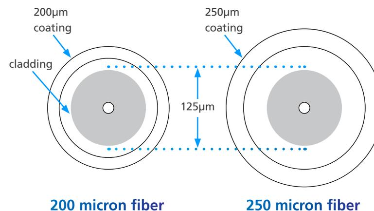
For optical performance and splice compatibility, 200-micron fiber features the same 125-micron core/cladding as the 250-micron alternative. Source: ISE Magazine
