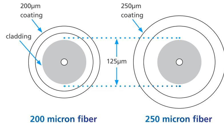
For optical performance and splice compatibility, 200-micron fiber features the same 125-micron core/cladding as the 250-micron alternative. Source: ISE Magazine
