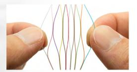
Rollable ribbon fiber is bonded at intermittent points. Source: ISE Magazine
