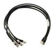
MQ Multiport cluster 5 ports cable assembly with interface type MQ female to 4.3-10 male,size 1/4", length 0.5 meters
