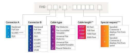
Cable Type K not available with LC & SC Options Cable Length shown as an example, additional cable lengths available upon request up to 2,000 ft. (600 m). \*\* \*\*\*
