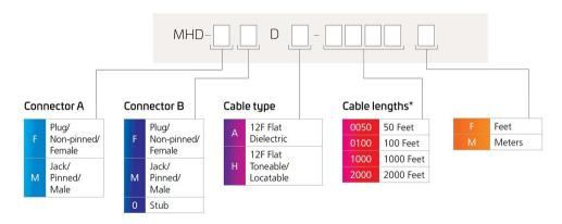
\* Cable Length shown as an example, additional cable lengths available upon request up to 2,000 ft. (600 m).
