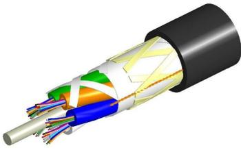
Fiber OSP cable, LightScope® ZWP All-Dielectric Self-Supporting, 72 fiber, 2.5mm Gel-filled Tubes, Singlemode G.652.D and G.657.A1, Meters jacket marking, Black jacket color
