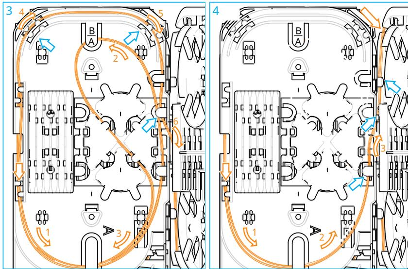
3 To route the feeder fibers coming from the uncut storage zone through the channels at the top side of the front tray, the fibers first need to make a U-turn through the channel in the island.
