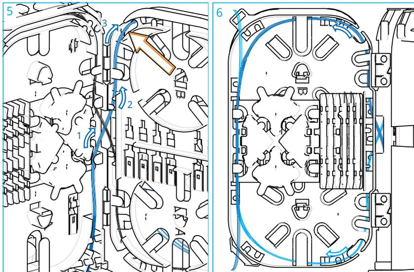
5 Drop fibers are routed through the slot at the top side of the hinged tray.
