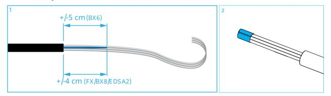
1 Prepare the cable as per standard practice. Cut the strength member at  $\pm$  5 cm (BX6) /  $\pm$  4 cm (FX/BX8/EDSA2) from the cable jacket.
