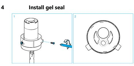
1 Before installing the gel seal in the port, install the 2 securing screws.
