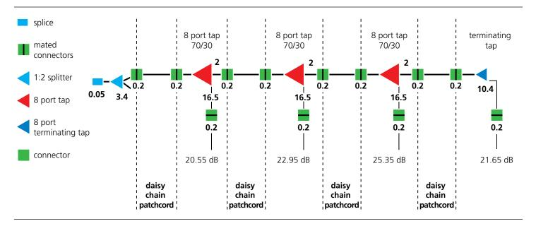
Hub: 0.05 dB (splice) + 3.4 dB (1:2 splitter) + 0.2 dB (hardened SC/ APC) = 3.6 dB
