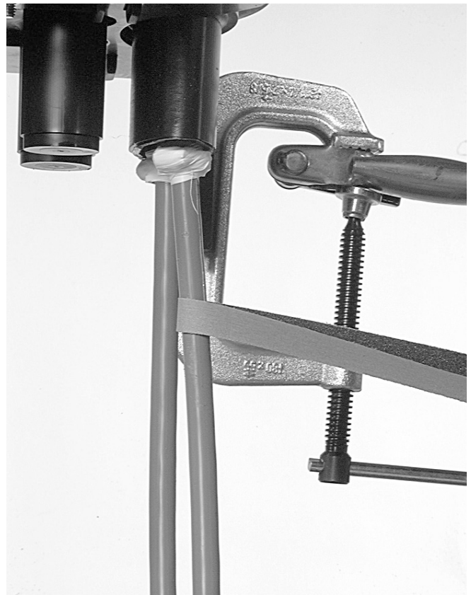
5.1.2 Clean and abrade the cable.
