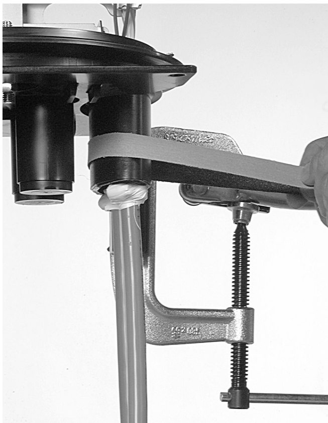
5.1.1 Clean by using the cleaning tissue. Abrade the port.
