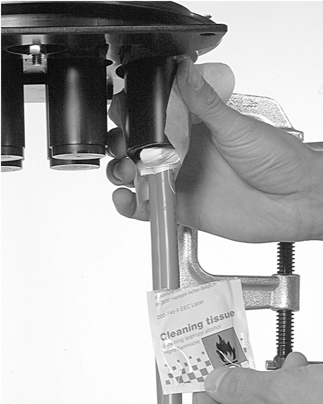
5.1.2 Clean and abrade the cable.
